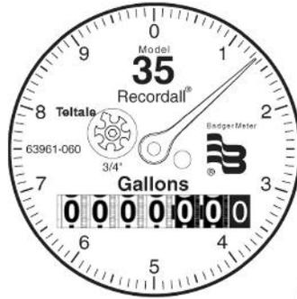
The 7 digit display at the bottom of the meter shows your current reading in tens of gallons. The needle shows from one to 10 gallons and provides the units digit when reading. The meter reading is not reset when it is read each month, but is recorded for use when the meter is next read.
